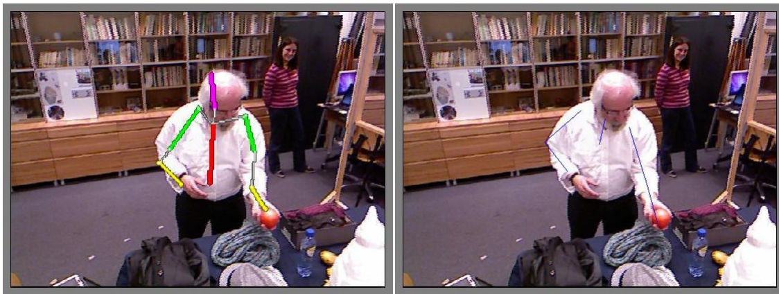
Figure 7.6: Limb detection comparison. Left: ETH tool. Right: Kinect.
