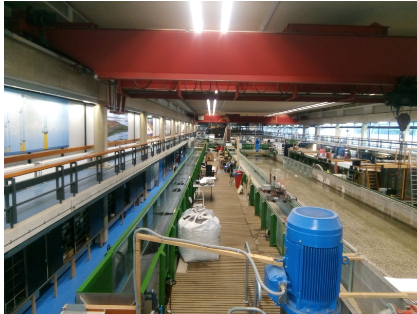
Figure 3.1: Wave Flume (left) and Sediment Flume (right) inside the Hydraulic Engineering Laboratory of TU Delft (TU Delft Faculty of Civil Engineering and Geosciences n.d.)
