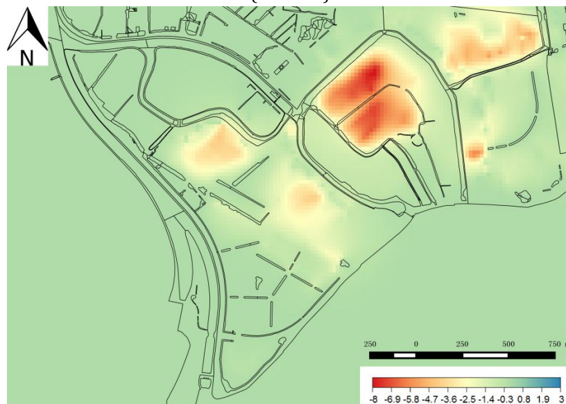
Figure 64 Change of mean groundwater level after adding 50% of amount to sewerage pipe conductance (Unit: cm)
