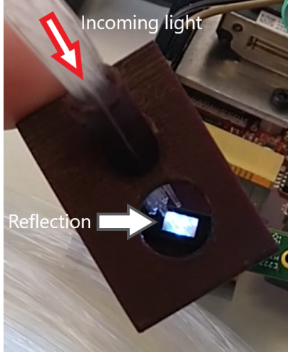
Figure 7: DMD reflecting light coming from optic fibers
