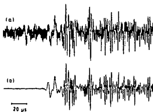
Fig 5.2 Noise reduction by signal averaging a) single shot b) same trace after 1000 times averaging
