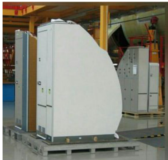
Fig. 1.02 Lavatory Monument exterior
