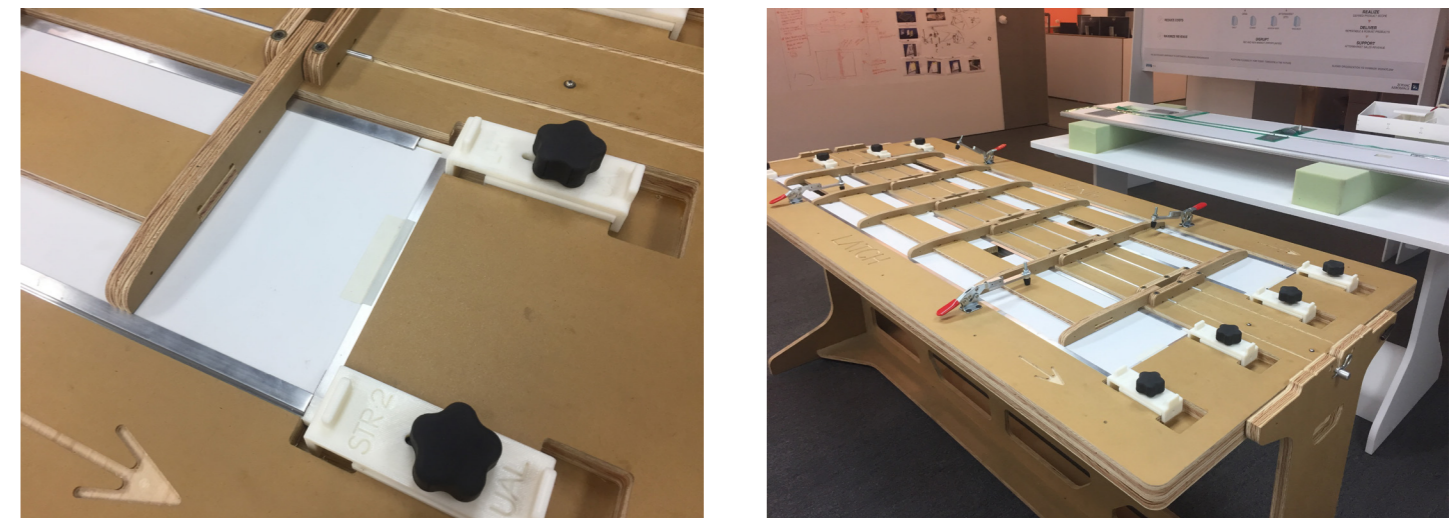
Fig.2.32 Tooling of a bi-fold door
