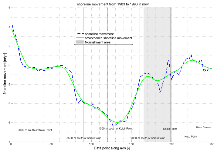
Figure 4-8: Shoreline movement from 1983 to 1993, derived from aerial photographs
