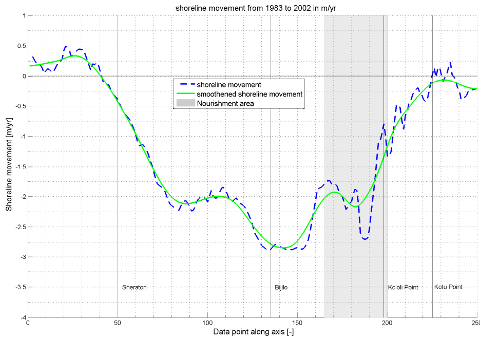
Figure 4-4: Shoreline movement from 1983 to 2002, derived from aerial photographs
