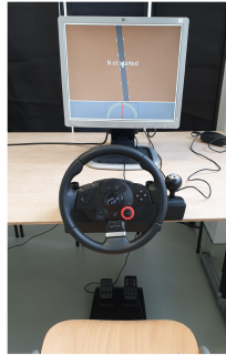
FIGURE 2. The experimental setup as seen from a participant's view. The other participant in the pair used an identical setup. The participants could not see each other.
