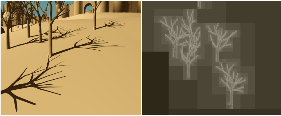
Figure 1.2: Left: A compressed multiresolution hierarchy is used to generate detailed shadows of trees. Right: The structure used encodes depth in a hierarchical manner, using smaller (deeper) nodes as needed. Nodes in deeper tree levels are shown in lighter colors.
