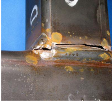
(a) Brace fracture in specimen CX1-40_420R [24]
