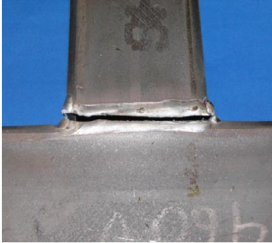
(b) Weld fracture in specimen CX1RT_460V [24]
