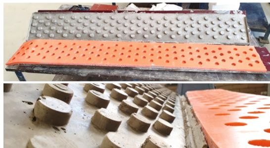
Fig. 2. Shearkeys in profiled SHCC laminates.
