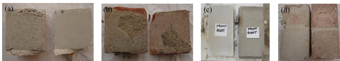
Fig. 13. Top view from the debonded surface of CS and clay masonry specimens: (a-b) cores; (c-d) triplets.
