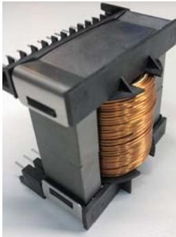
Fig. 5. The Prototype Td with displacement winding as Fig. 3 (d).
