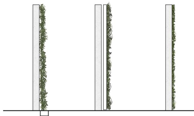
Figure 2 - Green wall systems. Left: green facade. Middle: living wall system. Right: bioreceptive facade.
