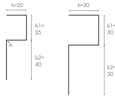
Figure 5.8- Dimensions rectangular section
