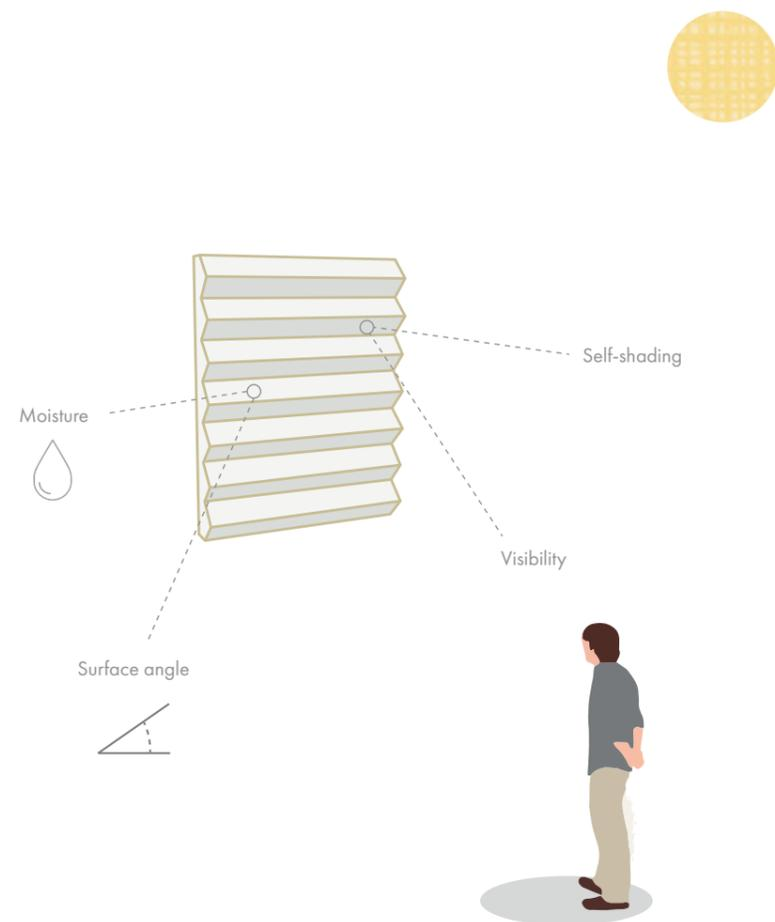
Figure 4.9 - Contradictory design factors for the panel design.
