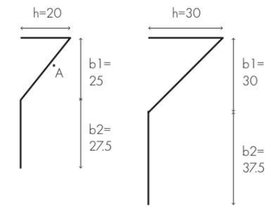
Figure 5.9 - Dimensions triangular section
