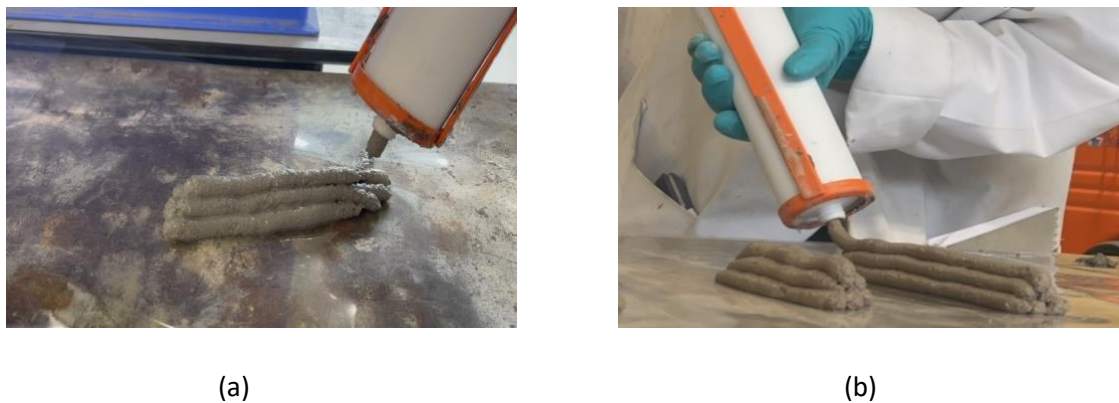
Figure 4.8 Mini extrudability test conducted on (a) reference mix (20FA-BFS_0.38) and (b) target mix (20BA-BFS_0.40).
