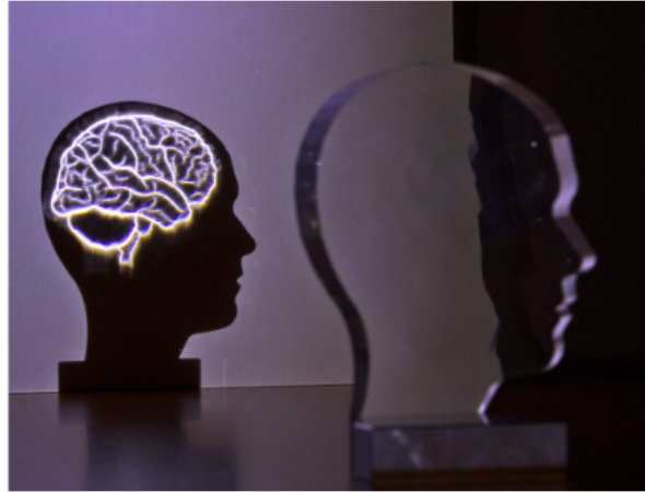
Figure 2.3.1: 'Caustic Brain': An example of caustic design. The transparent acrylic slab is designed to refract the incoming light into the shape of a human brain. Figure taken from [Schwartzburg et al., 2014].
