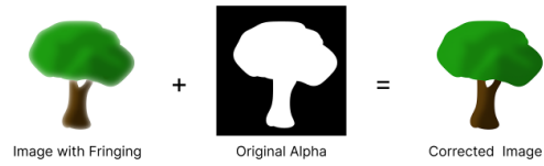
Figure 3: Diagram showing the fringing removal process. For alpha, white represents an alpha value of 1 and black represents 0
