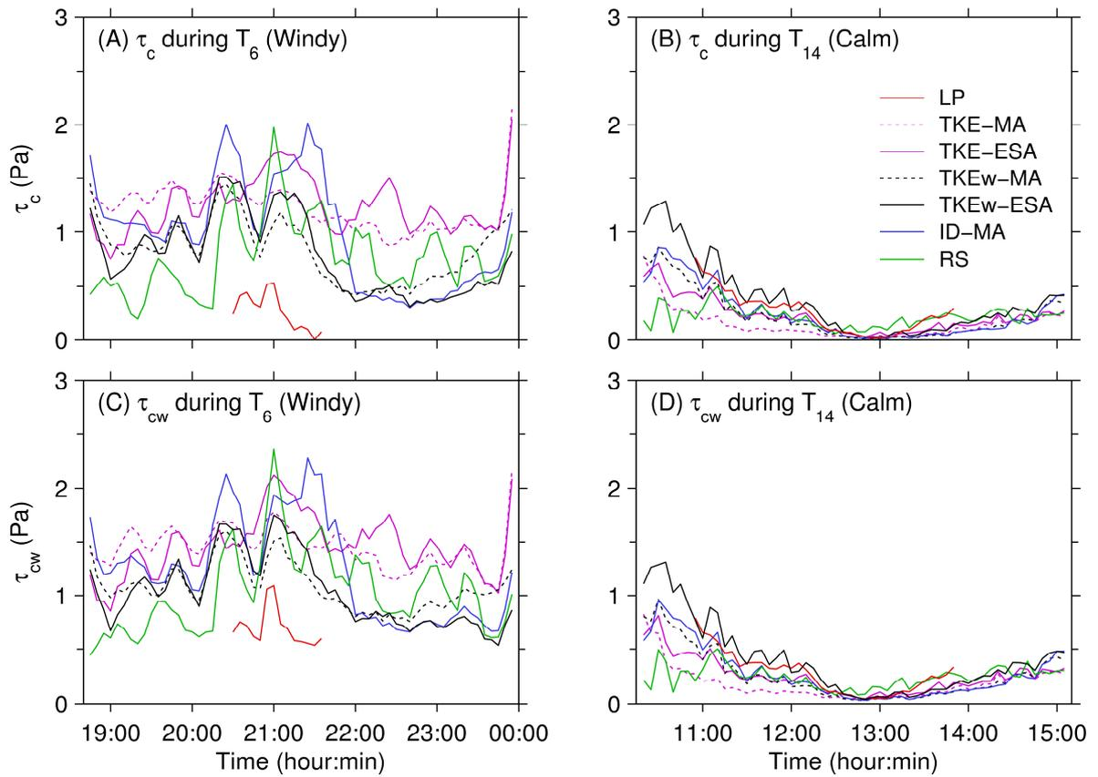
**Figure 6.** Expanded sections of the time series of  $\tau_c$  and  $\tau_{cw}$  obtained using the various approaches. The two tidal cycles are representative because tidal-average  $\tau_{cw}$  in the cycle in July 28<sup>th</sup> and August 1<sup>st</sup> reaches maximum in windy period and minimum in calm period, respectively. Legends in panels (A), (C) and (D) are the same as that in panel (B).
