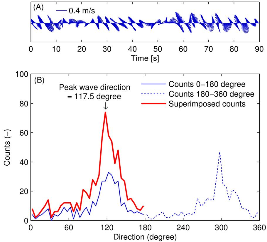
**Figure 2.** (A) Vector series of near-bottom wave orbital velocity filtered from the ADV in a burst, and (B) its direction (in Cartesian coordinates) count.
