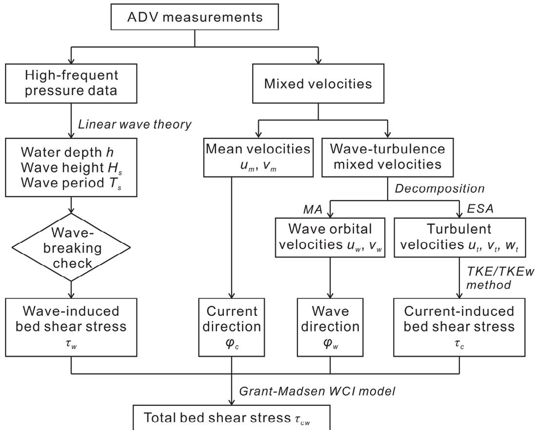
**Figure 8.** Protocols for estimating total bed shear stress under combined wave–current action,  $\tau_{cw}$ , using in situ ADV data.
