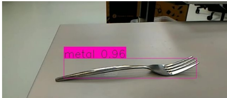
(b) Object detection algorithm output displaying the detected materials and its confidence score.
