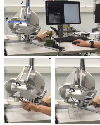
Fig. 4. Photos from the experiments. The photo on the top shows the human operator controlling the slave robot through the master device (computer mouse). The photo on the bottom left shows the position tracking experiment. The human assistant applies physical perturbations on the end-effector of the robot. The photo on the bottom right shows the contact establishing experiment. The robot base frame orientation is illustrated by the blue arrows for y-axis and z-axis. The x-axis follows the right-handed coordinate system.
