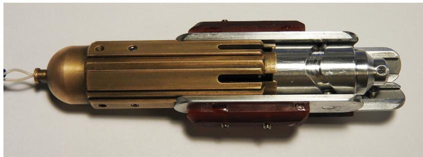
**Figure 48:** Photograph of the the sliders which move within the path that is milled into the barrel cam.
