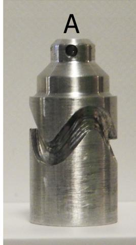
**Figure 60:** Photograph of the barrel cam that provides the bisected reciprocating motion.
