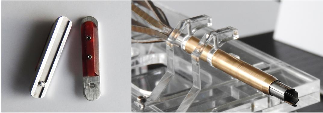
**Figure 46:** Photograph of two 3D-printed plastic blade adapter clamps glued to sliders (left). One of the sliders is turned upside down in order to display the ball bearing which follows the path on the barrel cams. In addition, a the configuration of the blades within the milled brass tube is shown (right).
