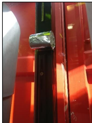
Figure 44 Placement of an aluminium casing around the sensor
