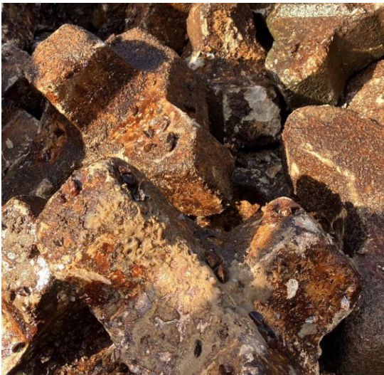
Figure 6.11: Xstream blocks that were retrieved from a groyne in the pilot project 'Flexible groyne show clearly that species have colonized the elements (Buschman et al., 2024).
