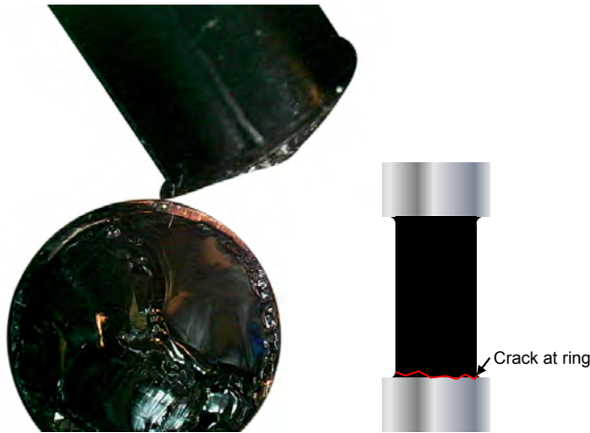
Figure 4.15 Example of brittle fracture of reference specimen broken near the ring; at the right a schematic indication of the location of crack interface, at the left a photograph of both crack interfaces; at the top the side view of the column is shown, at the bottom the top view of the fracture interface is given with the metal ring visible.
