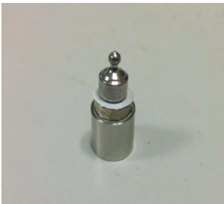
Figure 3.9 An assembled test specimen with a weight of 1 gram placed on top.
