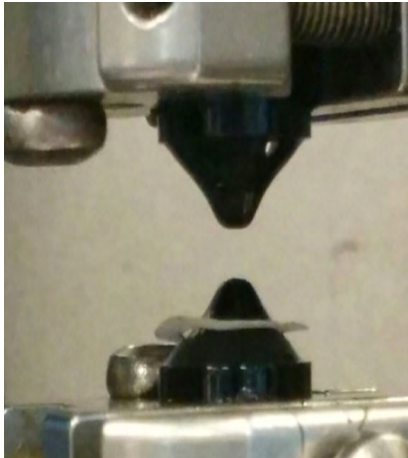
Figure 4.9 Healed specimen after the completion of a tensile test
