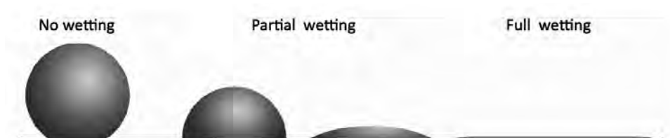
Figure 2.29 Possible interactions between a surface and a liquid. [By MesserWoland, https://commons.wikimedia.org/w/index.php?curid=1253800 ]
