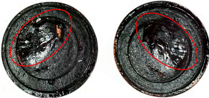
Figure 5.27 Surfaces of the top and the bottom half-specimens after tensile testing, storage healing, penetration grade 10/20, healing period: 16 hours, load: 10 gram, specimen 2, red circle indicates healed area.
