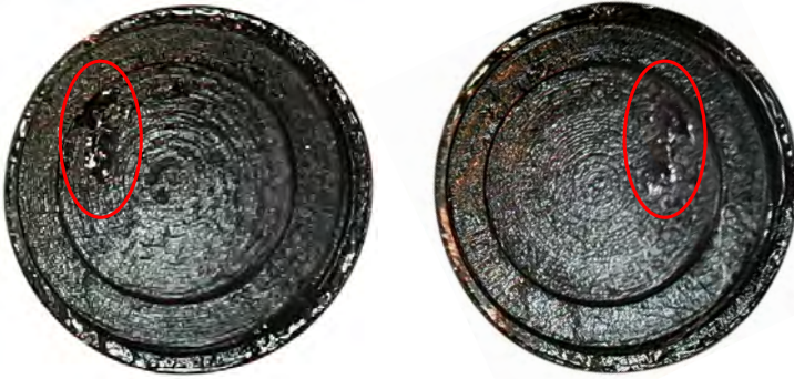
Figure 5.26 Surfaces of the top and the bottom half-specimens after tensile testing, storage healing, penetration grade 10/20, healing period: 16 hours, load: 1 gram, specimen 1, red circle indicates healed area.
