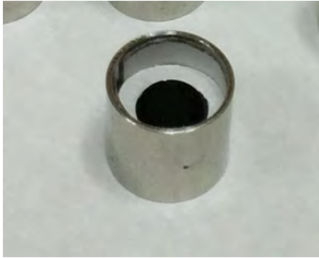
Figure 3.8 A half-specimen in the alignment tube with the silicon paper controlling the contact area visible on top.
