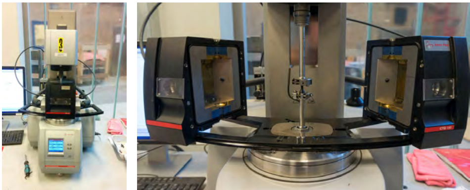
Figure 3.2 Anton Paar, EC Twist 502. Left: an overview of the machine, Right: with the oven open showing testing chamber and clamps.
