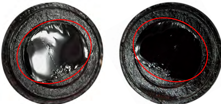
Figure 5.28 Surfaces of the top and the bottom half-specimens after tensile testing, storage healing, penetration grade 10/20, healing period: 168 hours (1 week), load: 1 gram, specimen 1, red circle indicates healed area.
