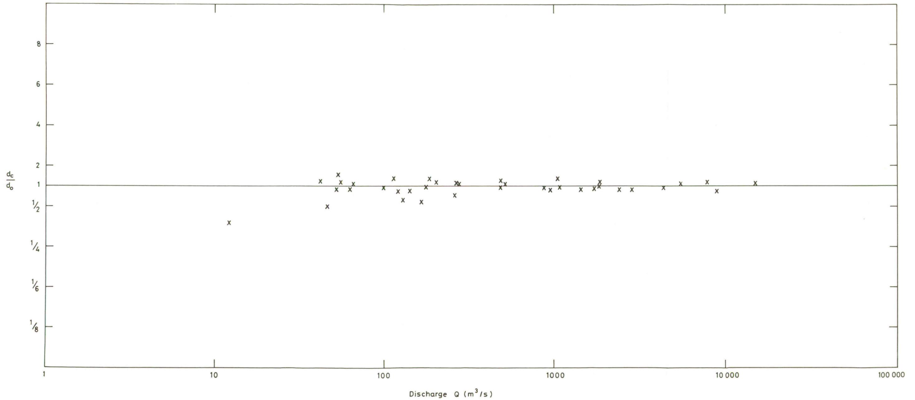
Discrepancy ratio for depth using observed slopes, gravel rivers
