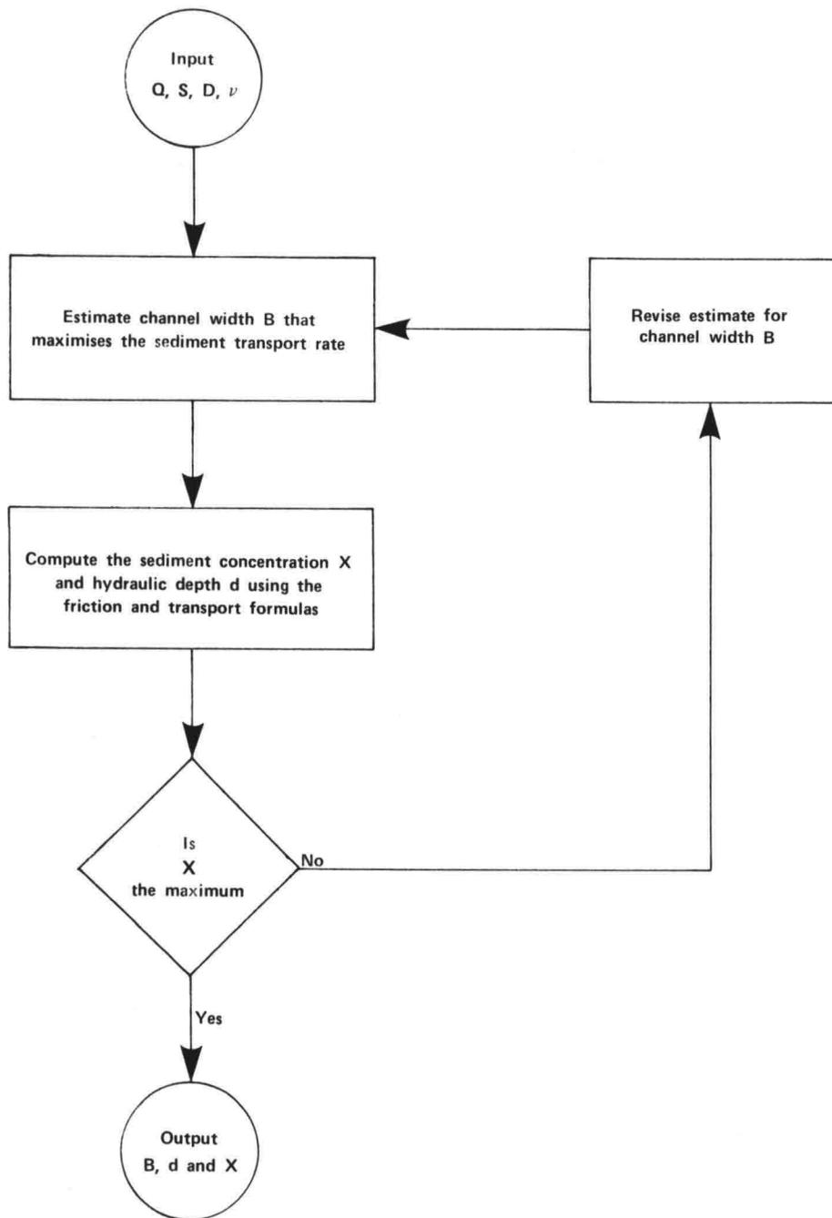
Flow chart for calculating maximum sediment concentration
