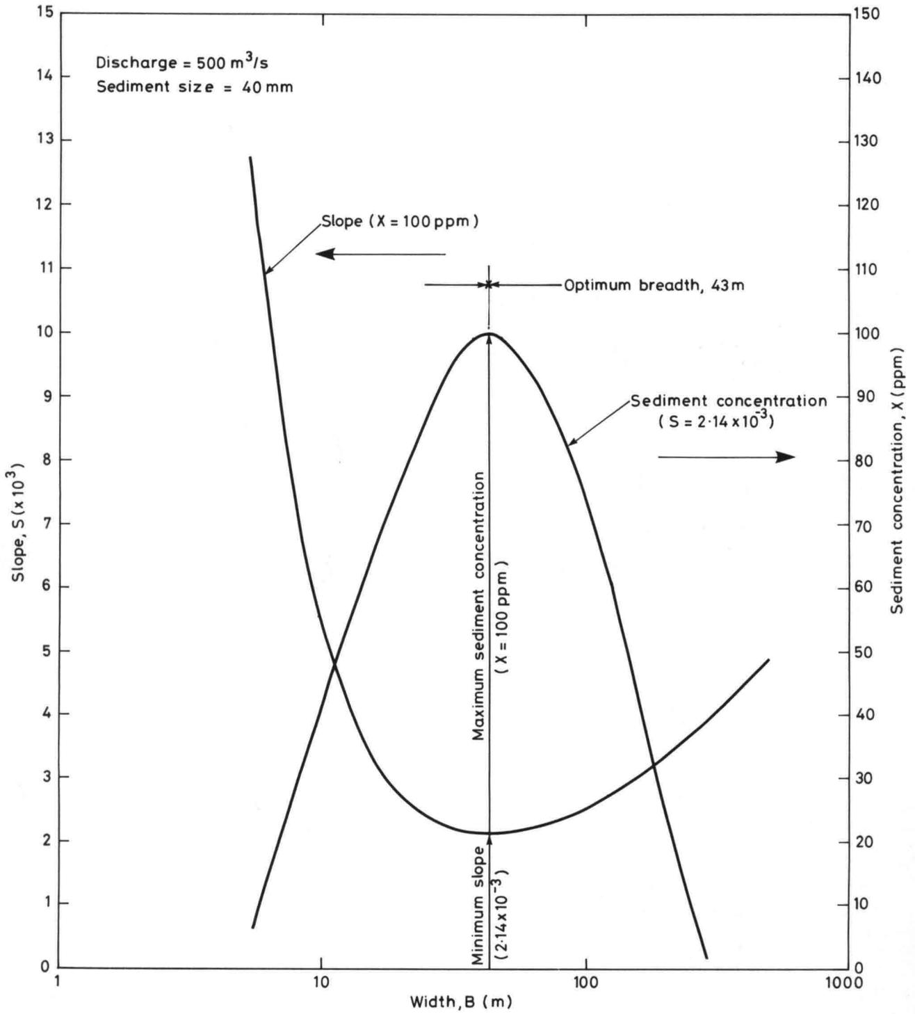
Slope and sediment concentration against width
