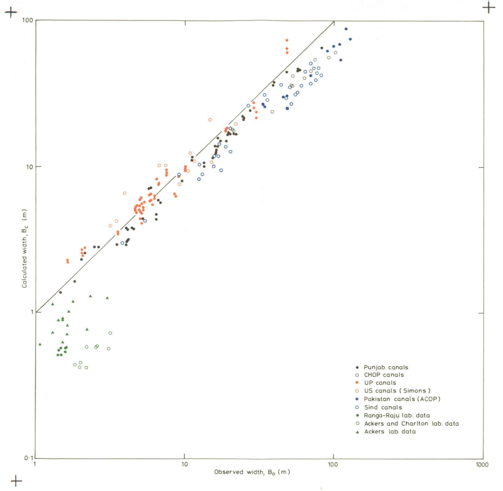
Calculated against observed width using observed slopes, sand channels
