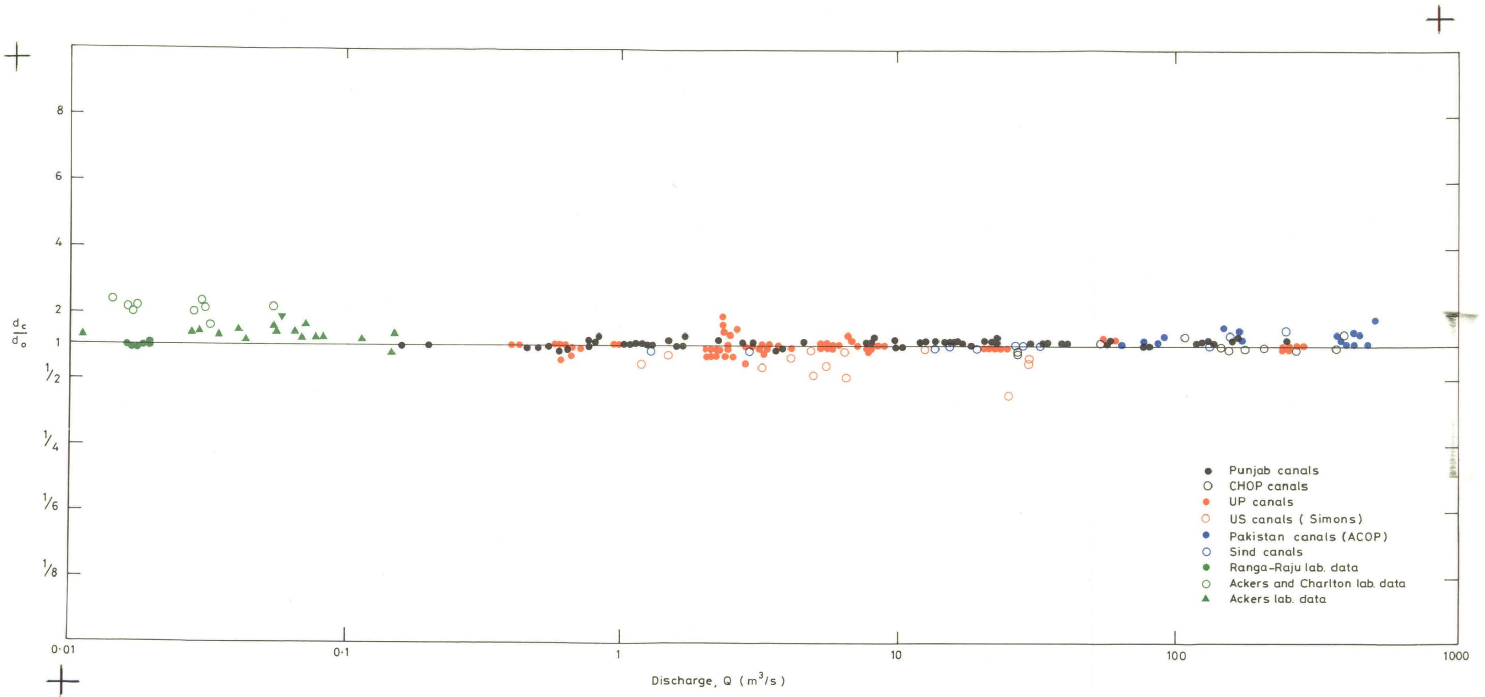
Discrepancy ratio for depth using observed sediment concentrations, sand channels
