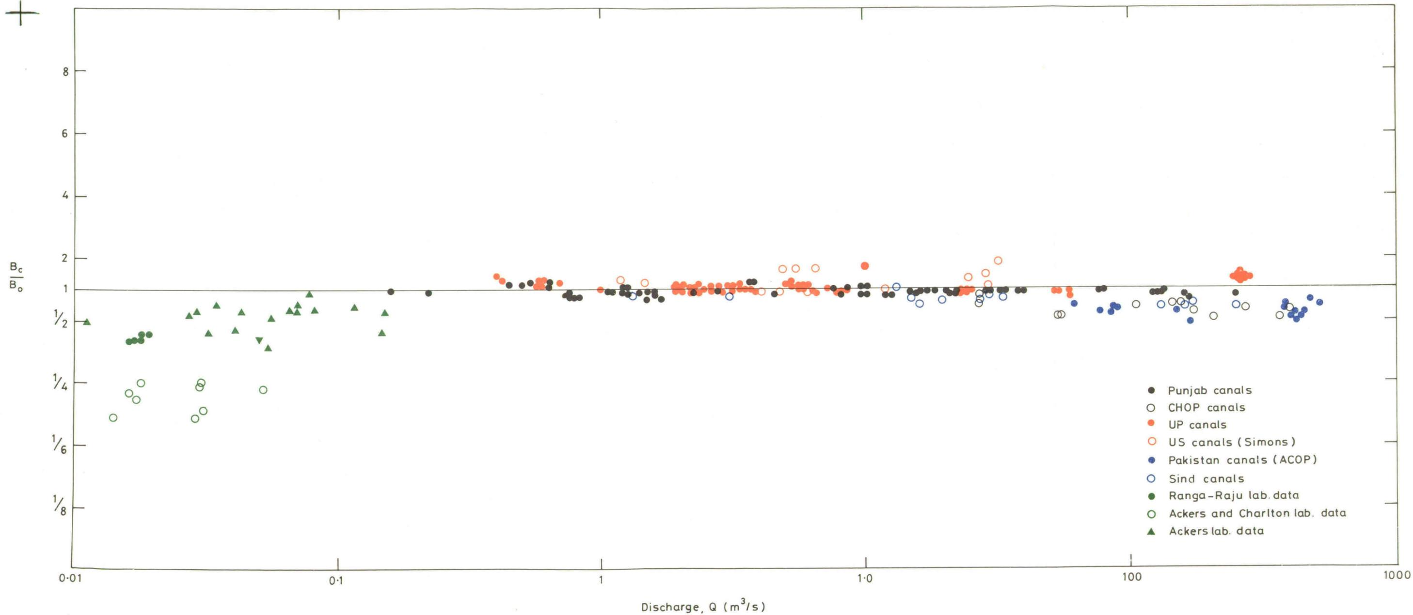
Discrepancy ratio for width using observed sediment concentrations, sand channels
