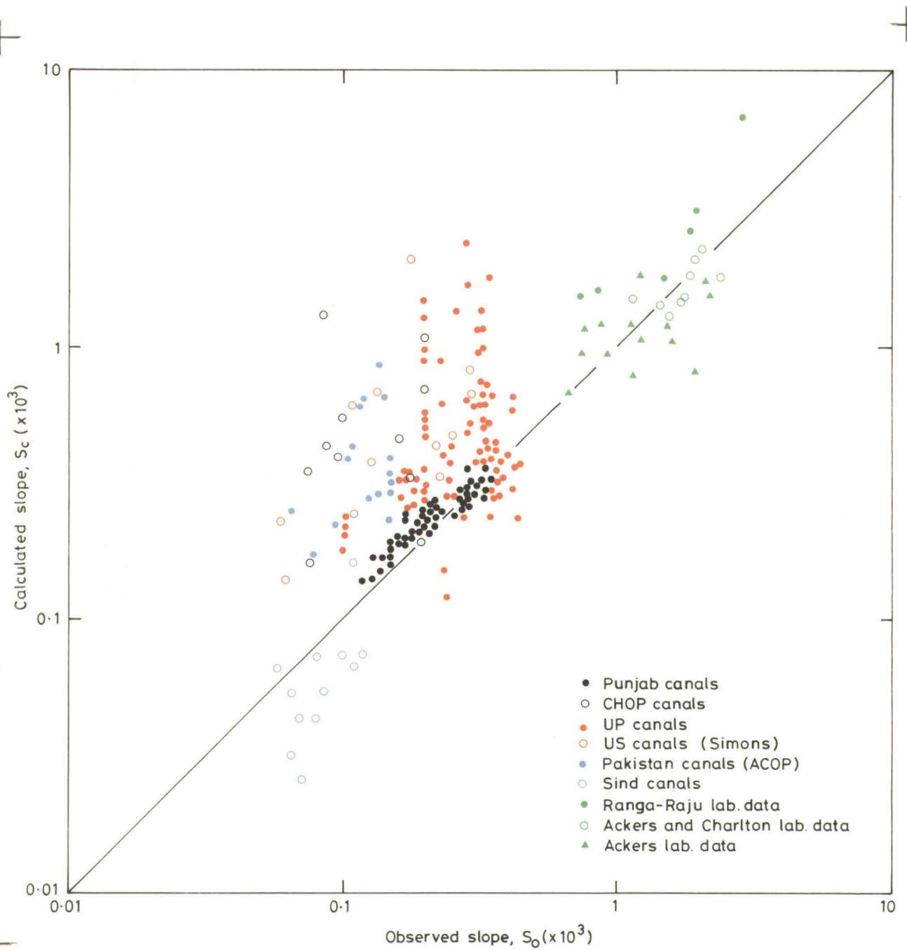
Calculated against observed slope using observed sediment concentrations, sand channels
