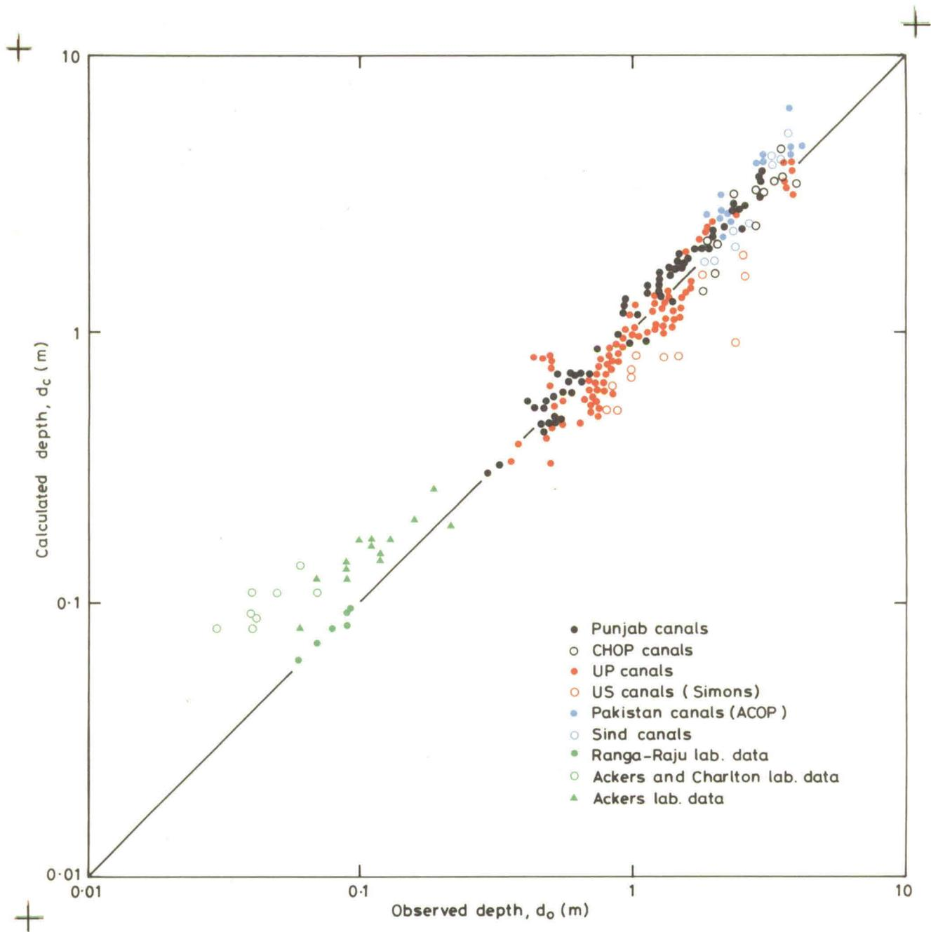
Calculated against observed depth using observed sediment concentrations, sand channels
