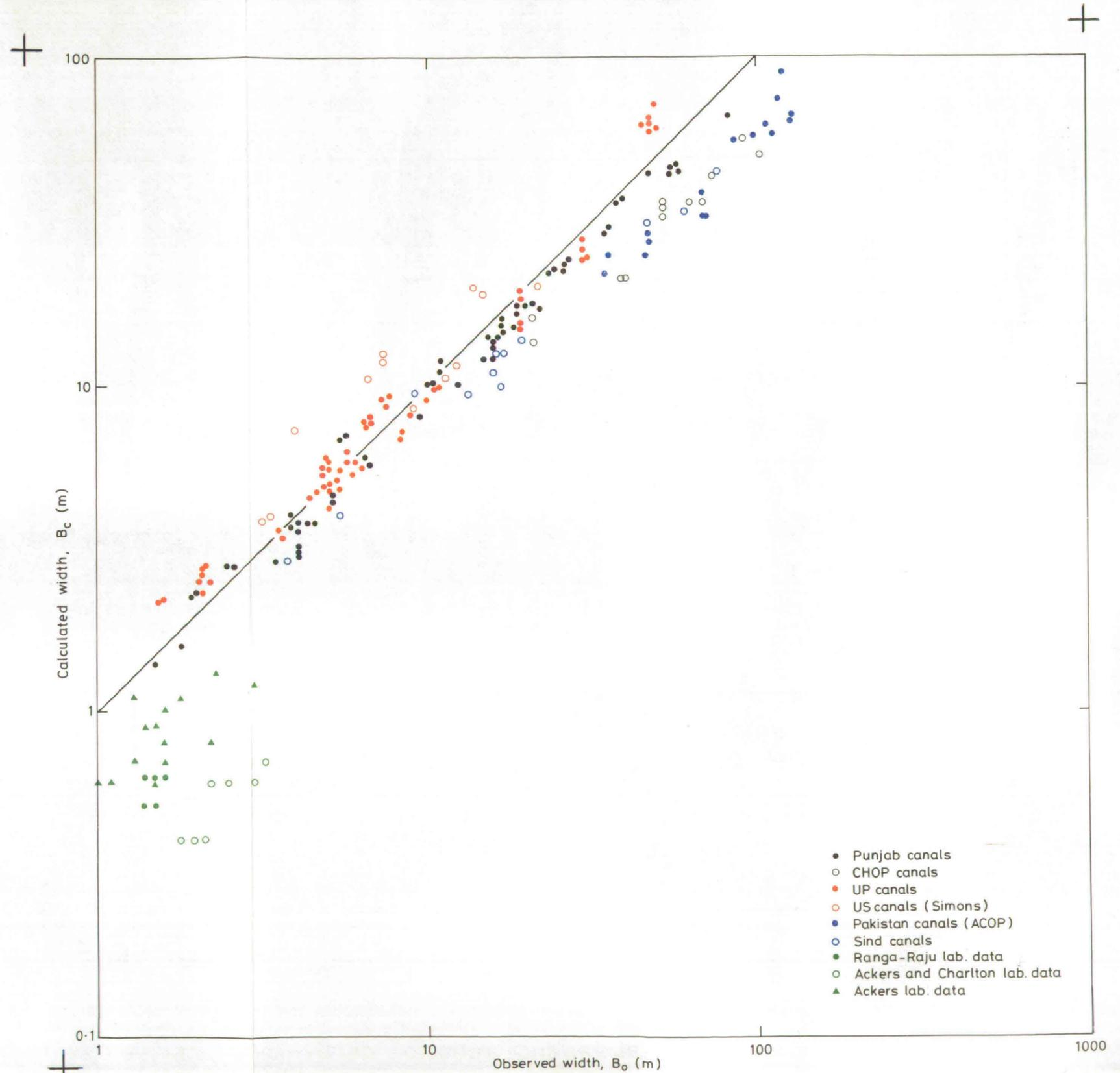
Calculated against observed width using observed sediment concentrations, sand channels
