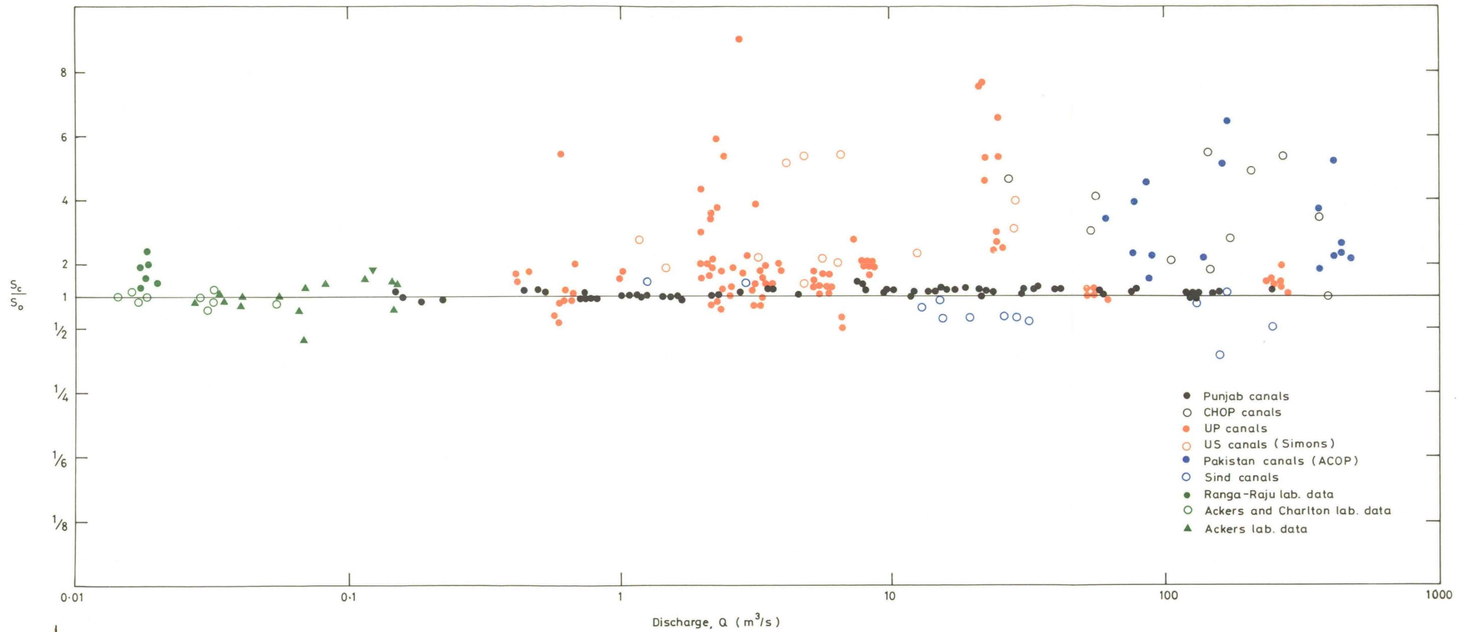
Discrepancy ratio for slope using observed sediment concentrations, sand channels
