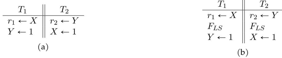
Figure 1.4: Two concurrent programs. (a) without Load-Store fences, (b) with Load-Store fences.
