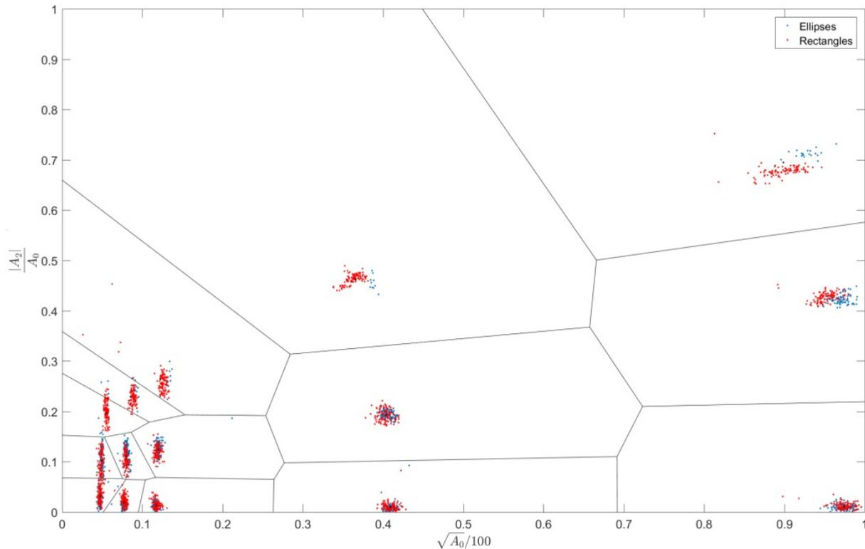
Figure 2 Scatter plot of the 2<sup>nd</sup> order versus 0<sup>th</sup> order Fourier coefficient of the scatterometry data for the 3000 programmed defects as defined in Table 1. Each cluster of data points can be related to a class within the set of programmed defects, e.g. the 3 clusters at the far left correspond to the 60-nm defects with aspect ratios of 1, 2, and 5 from bottom to top.
