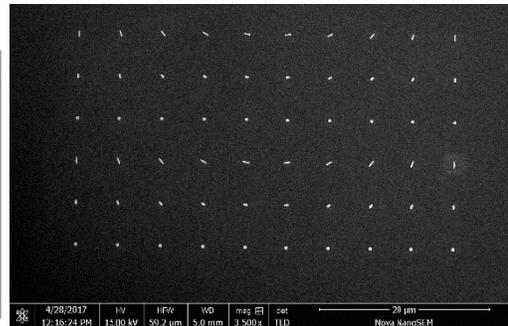
The detection step for these programmed defects was skipped as the location of the defects was already known from the sample design. The design coordinates of all defects were transformed to the stage coordinates of the Rapid Nano by finding the stage coordinates of 3 markers on the wafer. Optical defect review was performed for all 3000 defect locations.
