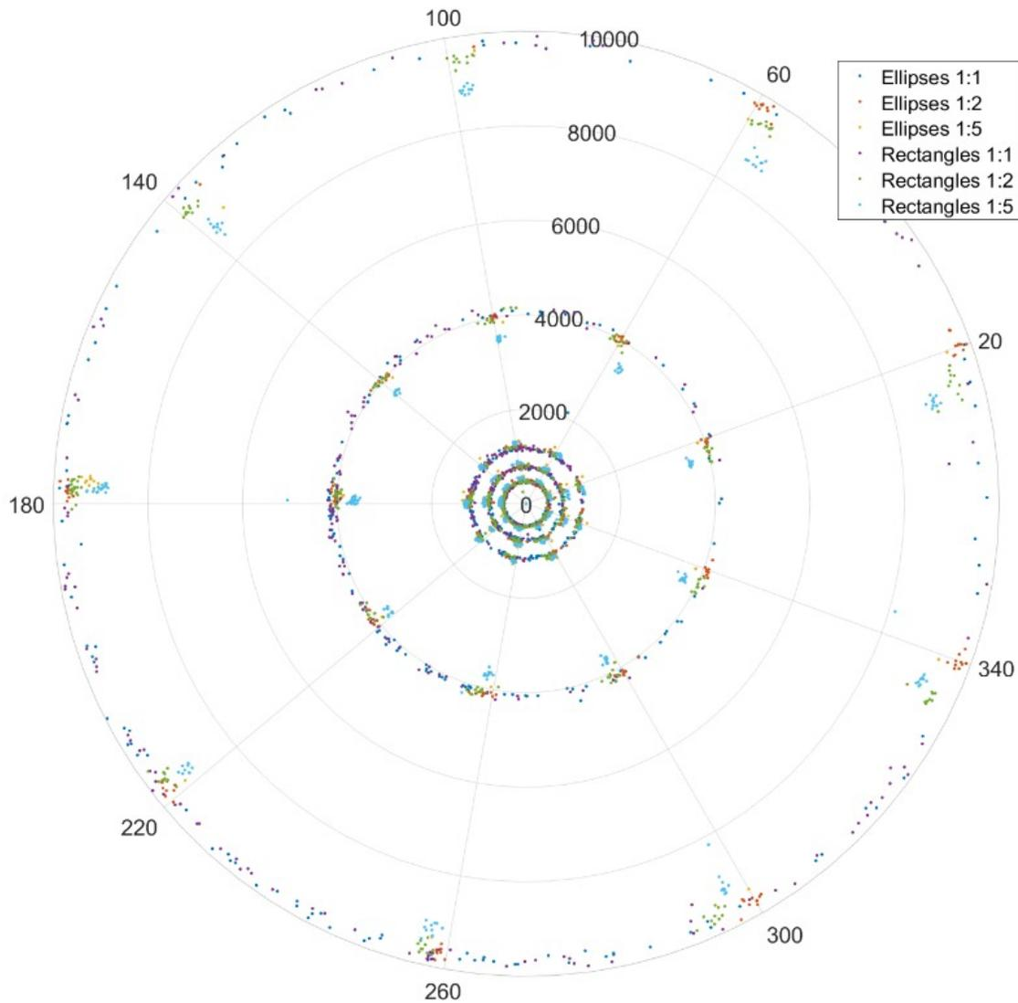
Figure 3 Polar plot of the RN3.9 signal (gv/J) versus the phase of the 2<sup>nd</sup> order coefficient  $A_2$  of the Fourier transformed scatterometry data for the 3000 programmed defects as defined in Table 1. Defects of similar size but with a different shape show up at approximately the same radius. Defects with a clear orientation show up at the corresponding angle.
