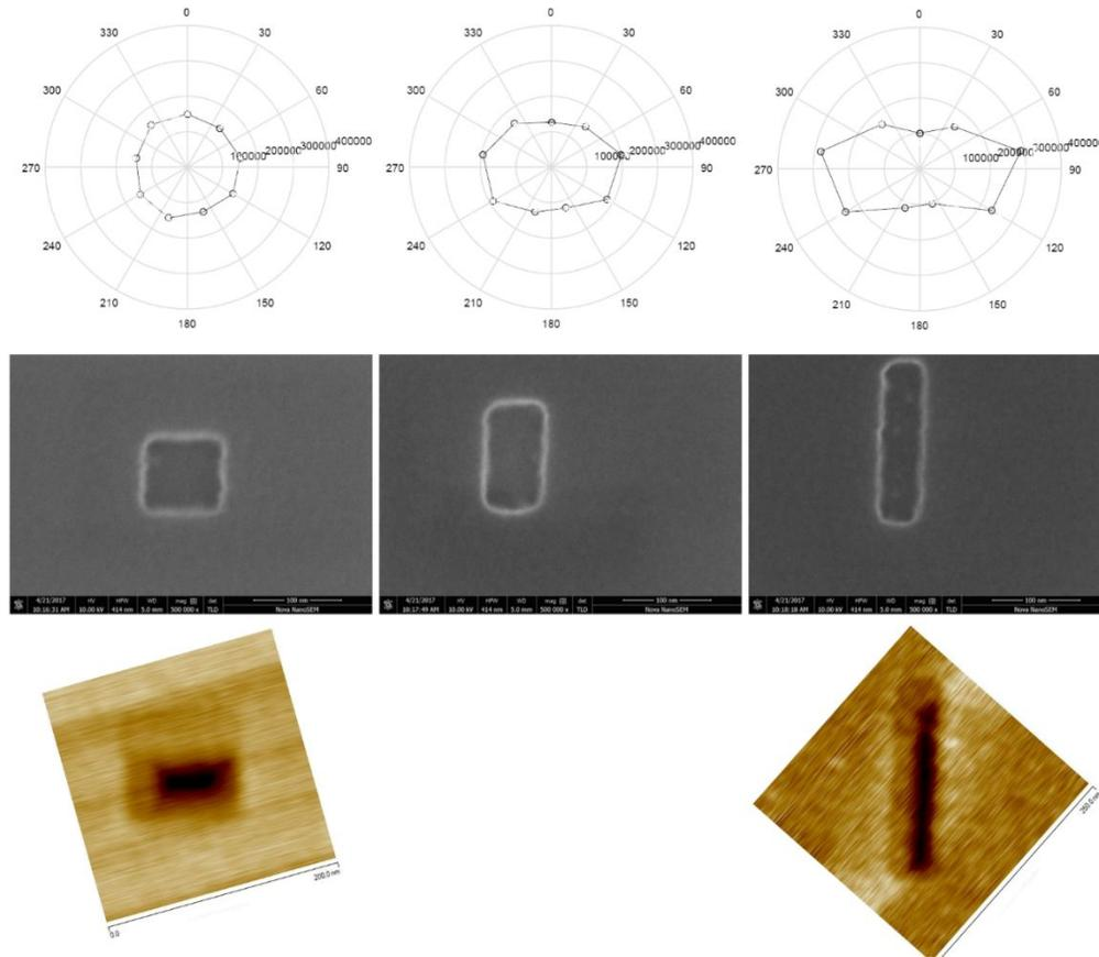
Figure 1: Optical signal strength (gv/J) as measured using RN3.9 for 9 angles distributed around 360 degrees scattering directions (top row) and SEM (center row) and AFM (bottom row) images, all from the same re-detected programmed defects. The design size of the square defects is CD = 100 nm, with aspect ratio AR = 1:1 (left column), 1:2 (center column) and 1:5 (right column). The defect volume is kept constant.
