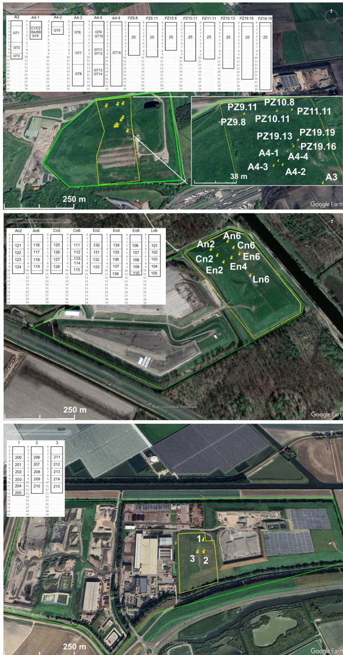
Figure 4.1: Aerial photographs (Google earth) of the pilots (green line), in situ stabilization landfill pilots (yellow line), and schematic (top left in each subfigure) showing the waste samples depth. Top: Kragge II; middle: Braambergen; bottom: Wieringermeer.
