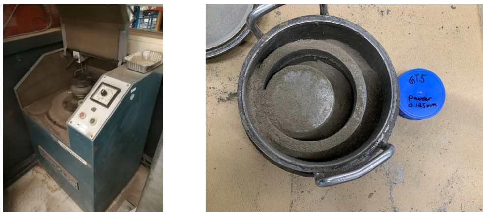
Figure S4.2.2.4: Herzog HSM 100 P disk mill (left). Milled sample in the disk mill container (right)
