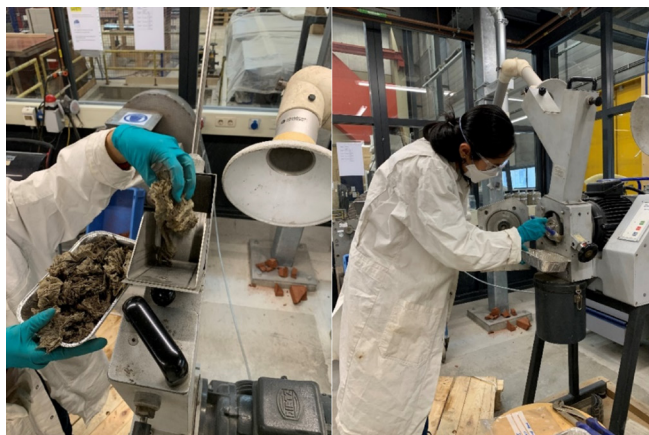
Figure S4.2.2.2: Left: inserting sample into the milling machine. Right: collecting the sample with a brush
