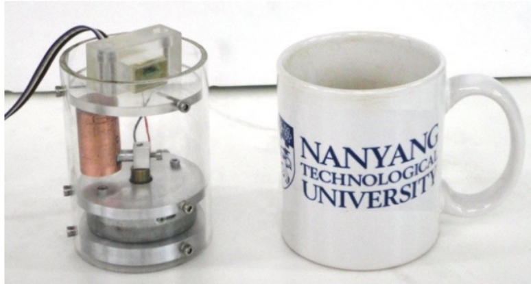
Figure 3.12: Smart Mug, an ergonomic hand-held design to measure arm impedance
