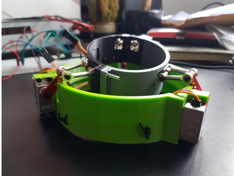
Figure 6.20: Loss of parallelism due to singularity
