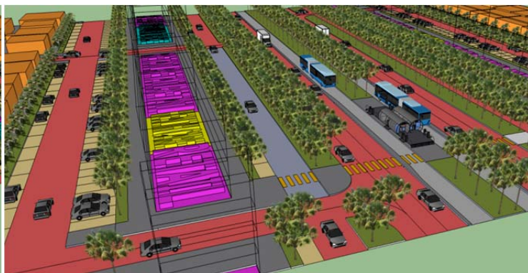
Figure 104: Closer 3D view from the same direction showing the overpass bridge and the transfer station building organization.
