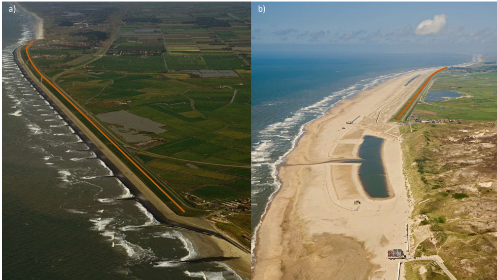
Figure 2.1.: a) Hondsbossche sea dike before placement of the nourishment (courtesy of Rijkswaterstaat, https://beeldbank.rws.nl/ , accessed on 6 September 2021) and b) the Hondsbossche Dunes Nourishment just after placement in April 2015 (courtesy of Aannemerscombinatie Zwakke Schakel–Van Oord-Boskalis). The orange line marks the crest of the original sea dike.
