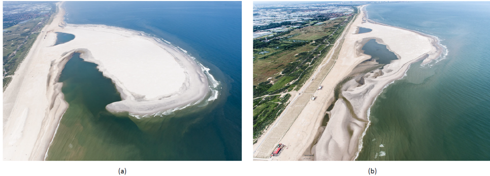
Figure 4.1.: Aerial photos of the SE, taken from the North, in a) July 2011 (shortly after construction) and b) July 2012 (after the first year). Source: Rijkswaterstaat and van Houdt (2012)
