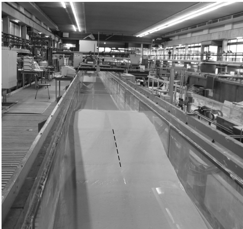
Figure 5.3 The barrier in the wave flume looking towards the sea
