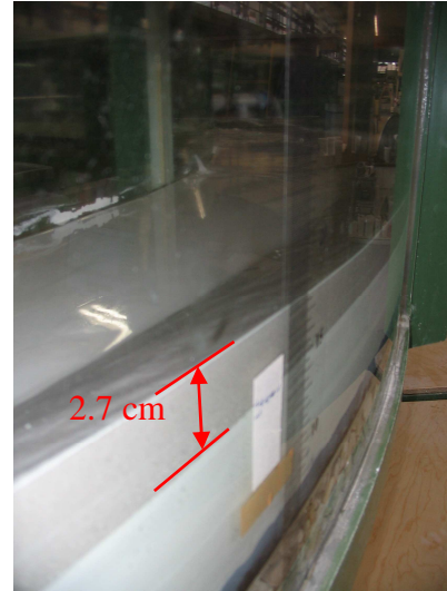
Figure 4.13: Picture taken at the outer wall after the test showing the sand accumulation on the bed surface in the corner along the outer wall. The height of the accumulated sand is shown.
