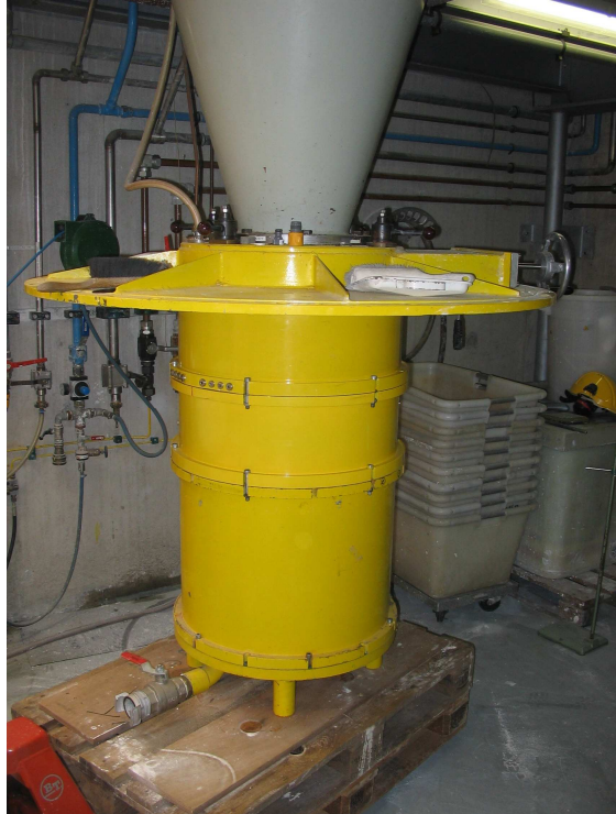
Figure 3.4: The yellow cylindrical container contains the sediment sample after the mixing procedure. The sample is transferred under gravity from the mixer into this container.
