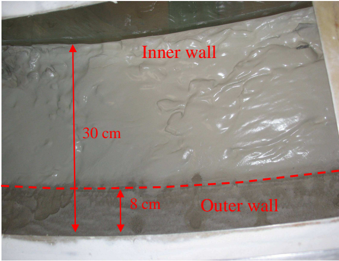
Figure 4.12: Top view of the bed surface after erosion. The accumulated sand along the outer wall is clearly visible. Also the holes in the sediment bed are shown.
