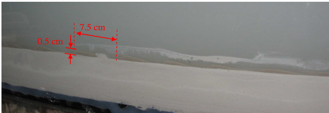
Figure 4.11. Picture taken at the outer wall of the flume showing sand ripples within the layer of accumulated sand. The ripples indicate bed load transport of sand. The average size of these ripples is shown.
