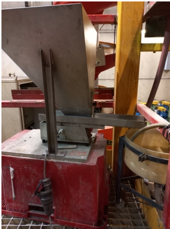
Figure 24. Feeding of the material to the shaking table (picture by Tero Korhonen)
