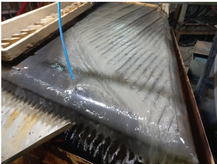
Figure 25. Gravity separation by the shaking table (Picture by Tero Korhonen)
