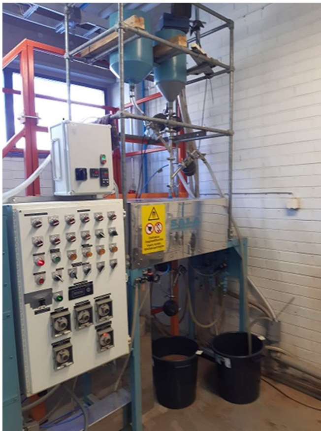
Figure 22. HGMS assembly in GTK Mintec (picture by Tero Korhonen)
