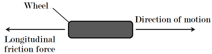
Figure 2.2: Force-body diagram for the longitudinal friction coefficient (adapted from Flintsch et al., 2012)
