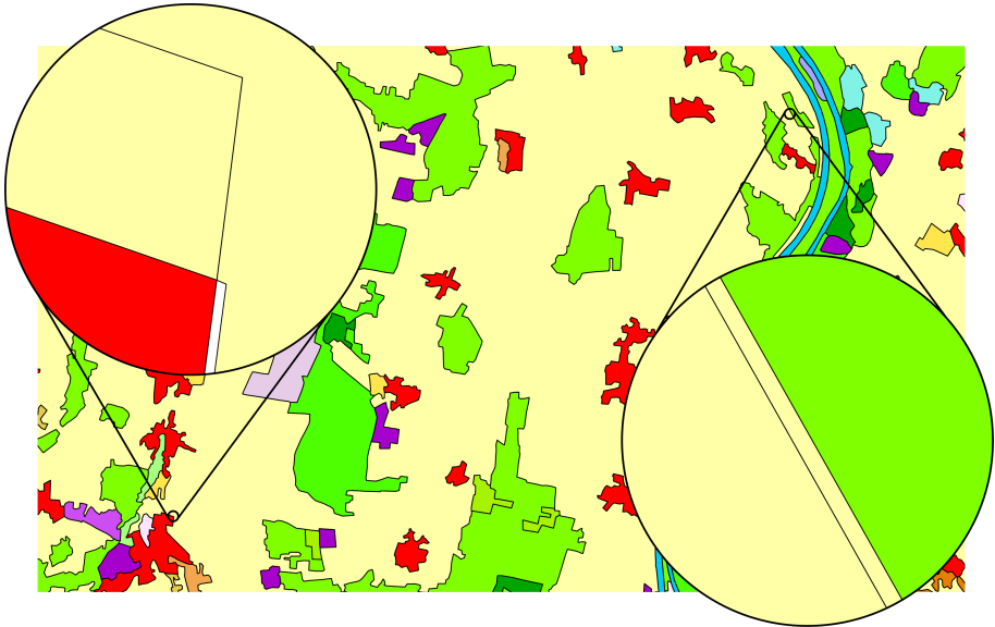
Figure 3.15: A polygon manually shifted (from CORINE2000 tile E41 N27) – it is overlapping with neighbours on one side and gaps are present on the opposite side (the size of the width of these gaps and overlaps is in the order of approximately 10 to 15 centimeter).
