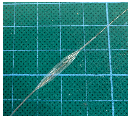
Figure 5.10: Balloon prototype with welded copper wire through balloon.
