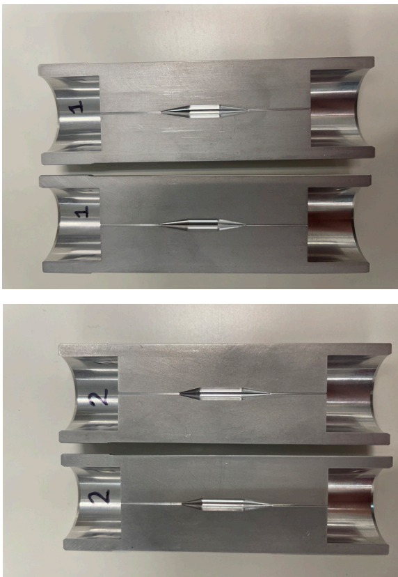
Figure 5.7 (left): Aluminum mold 1 for symmetrical balloon shape and aluminum mold 2 for the asymmetrical balloon shape.
