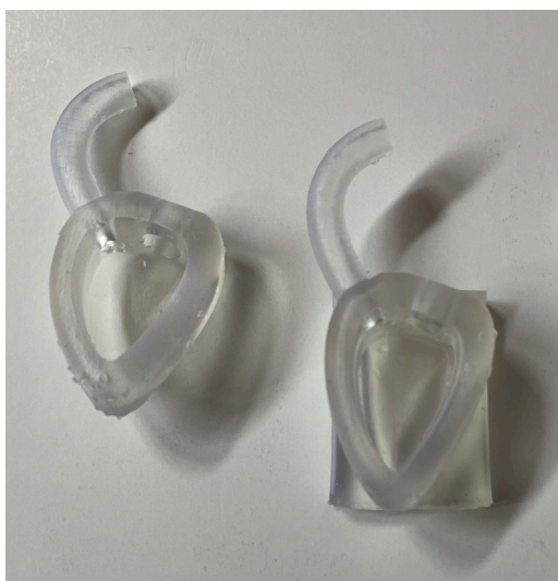
Figure H.2: 3D printed left ventricle models based on dimensions from literature. Without support square (left) and with support square (right).
