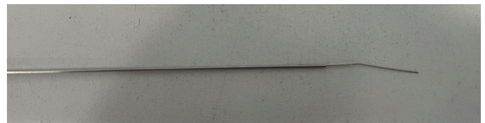
Figure 5.16: Prototype balloon advanced through 20G cannula
