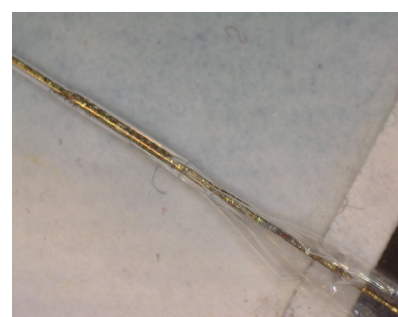
Figure 5.11: Microscope image of welded balloon tip with slight deformation at distal cone of balloon.
