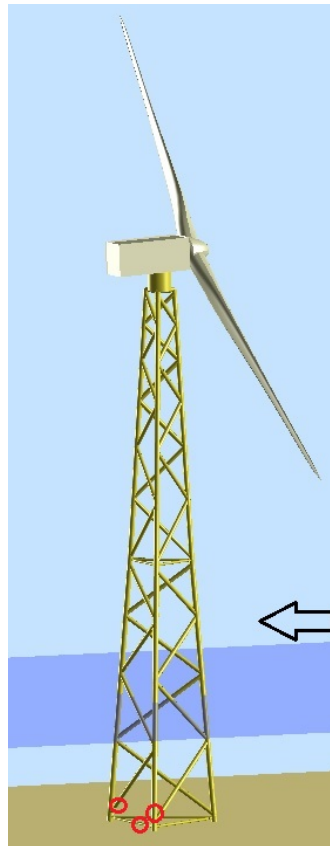
Figure 6-6: Location of the examined members on the structure. The red circles represent the points where the fatigue damage values were calculated and the black arrow shows the directionality of the loading. The RNA is wrongly displayed here, since it is a downwind model.
