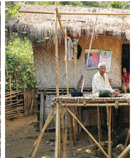
Fig. 115: House on stilts made of bamboo screens and thatch roofing
