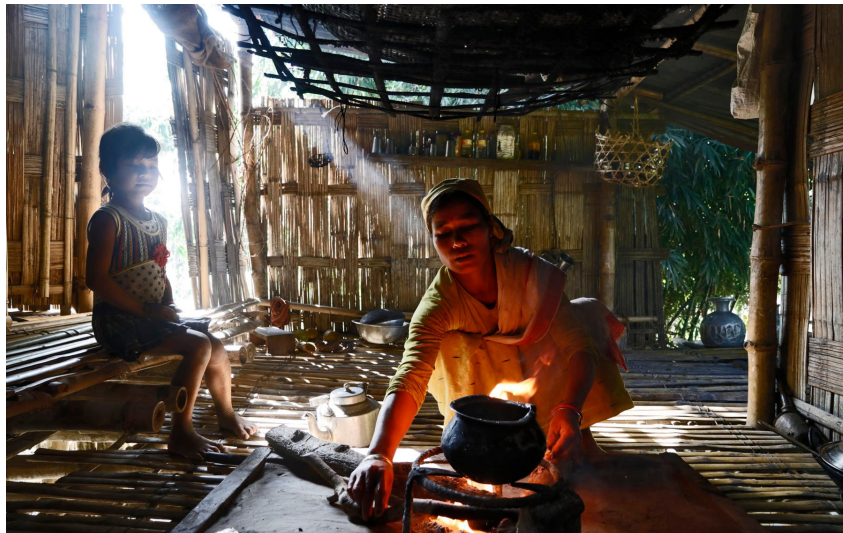
Fig. 112: The bamboo walls are not plastered, allowing natural ventilation in Assam's humid climate (Image © SEEDS / Siddharth Behl)
