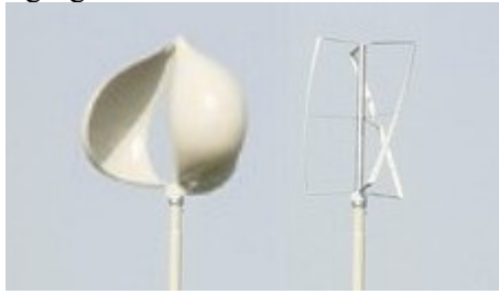
Figure 4 Example of two Vertical Axis Wind Turbines. Left, a drag-driven and right a lift-driven wind turbine.
