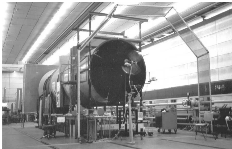
Figure 34 Overview of the open jet wind tunnel of Delft University of Technology during the experiments with a small H-Darrieus in skewed flow (Sardo [62]).
