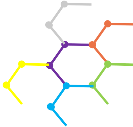
Figure 4.4: Hexagon enclosed in honeycomb structure, with only 3 individual links (Lines) and 2 joints (Circles).
