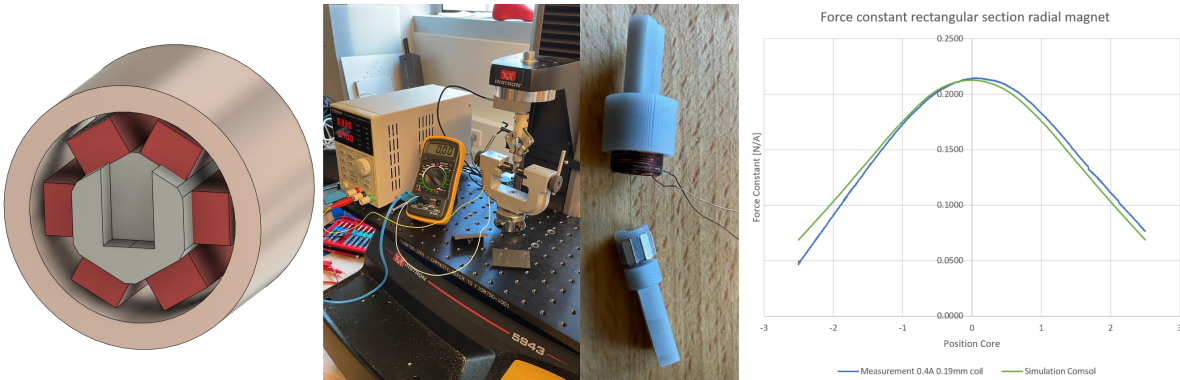
Figure 9.5: From left to right, actuator design, the manufactured prototype with its experimental setup and the measurement and simulation results.
