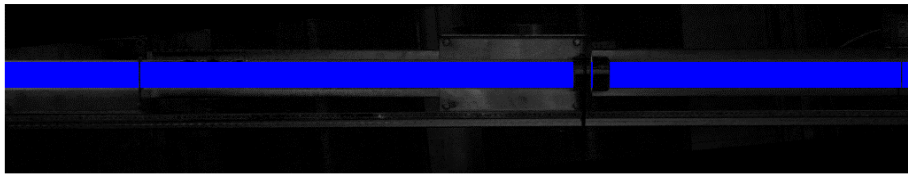
Figure 3.25: Part of image that is considered to be part of the pipe section.[20]
