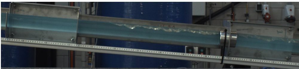
Figure 6.9: Last volume of oil, flushed from the pipe.
