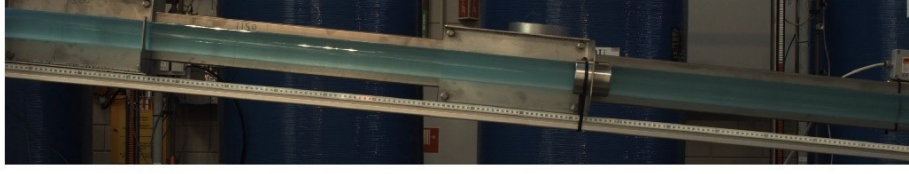
Figure 3.19: Water filled pipe at an angle of -5^\circ . [20]
