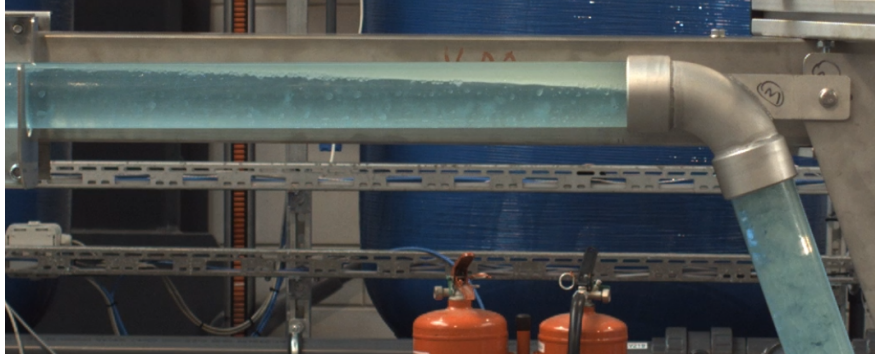
Figure 4.10: Oil residue stuck upstream of a sudden bend in the setup.
