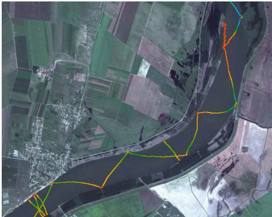
Figure 1.1. Scarce single-beam echo-sounder data. Cross-sections are formed when data are collected transversely of the river’s direction. “Trackline” data follow trajectories of the ships along a river (Danube River, Romania. Bing maps, 2015 ).
