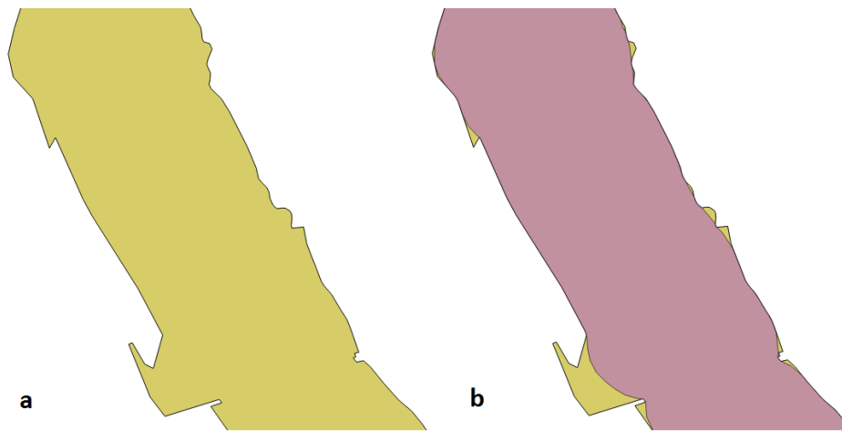
Figure 4.5. Simplification of polygon: (a) Original polygon, (b) Resulting polygon in purple after buffering-debuffering. Danube channel (detail, QGIS ).
