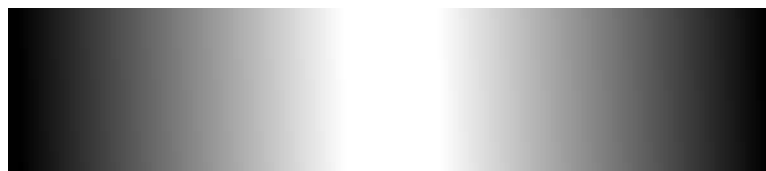
Figure 4.32. Gradient concept of weights applied in fusion method for cross-sectional scarce data. Black colour corresponds to the interpolated result, whilst white to the model computed topography.
