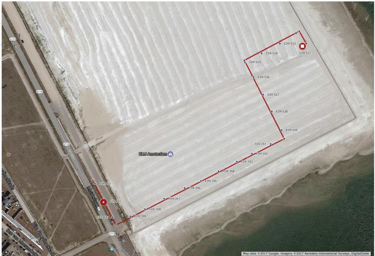
Figure 3.6 Locations of the CPT's for Centrumeiland IJburg (in 't Veld, Centrumeiland IJburg (onderheid transportriool), 2017)
