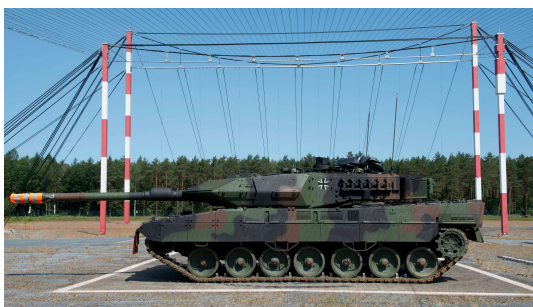
(a) A Leopard II placed in a bounded wave NEMP simulator owned by the Bundeswehr [5]
