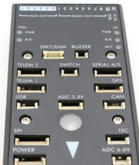
Fig. 7. The HobbyKing HKPilot32 micro-controller.
