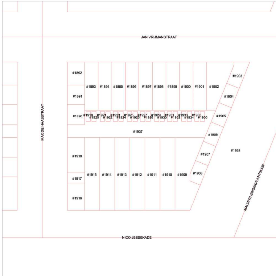
Figure 8: The part of the map accompanying the Kadasterwetthat is relevant for IJburg Block 44a. As can be seen, the land on which IJburg block 44a rests is divided into 28 plots and is surrounded by two larger plots: #1937 and #1938. Amsterdam leaseholds this land to its inhabitants.
