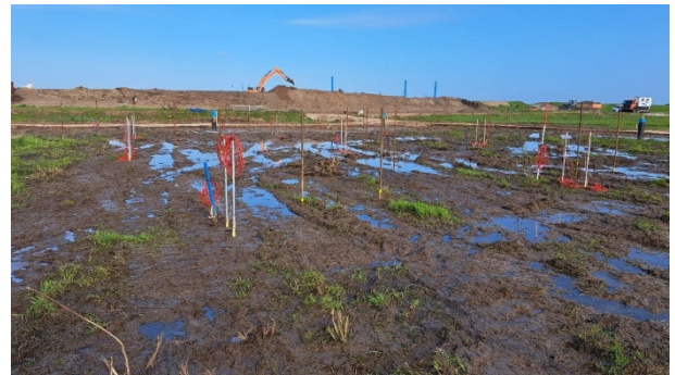
Figure 11. Photo of full-scale test with pore water pressure meters at the front.
