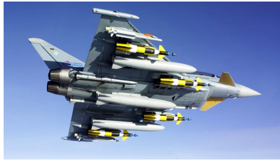
Figure 2.6: Example figure of a full armament Eurofighter store configuration. Image Credit: Creative Commons
