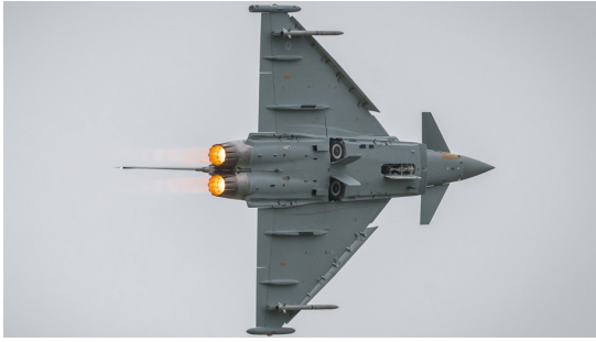
Figure 2.5: Example figure of an empty store configuration of the Eurofighter, comparable to the baseline configuration.
