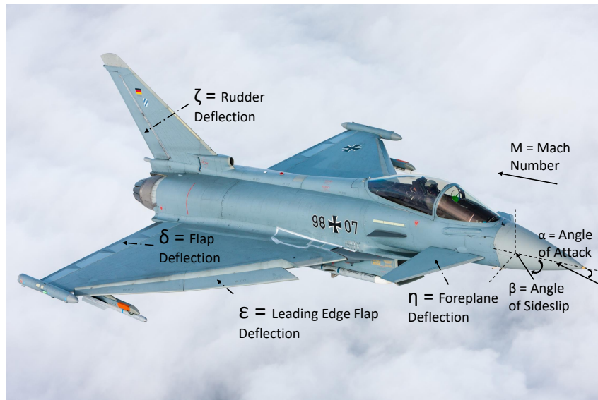
Figure 2.1: Image of a Eurofighter Typhoon in flight [2] with annotations of the control surface deflections and flow variables.
