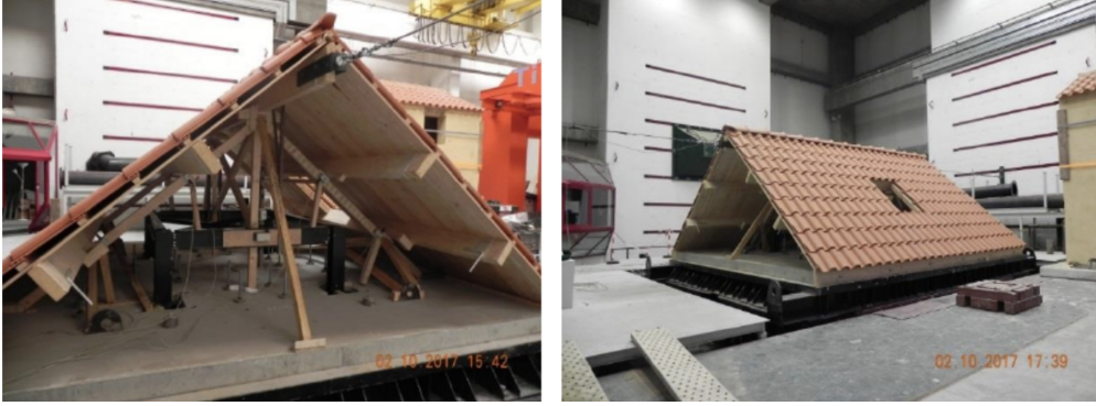
Figure 3.7: Replicated roof specimen from a terraced house tested at LNEC laboratories. From [147].
