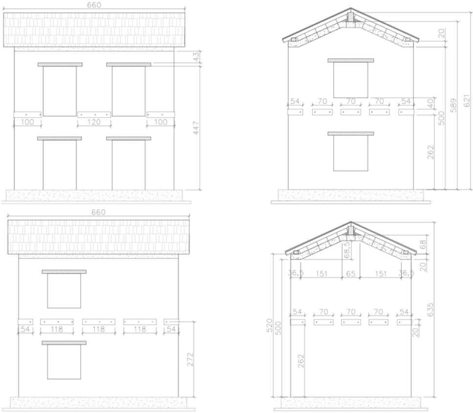
Figure 2.28: Full-scale building tested by MAGENES et al. [116]. Dimensions in cm.
