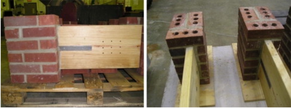
Figure 2.19: Side and front view of samples representing timber-masonry connections. From [54].
