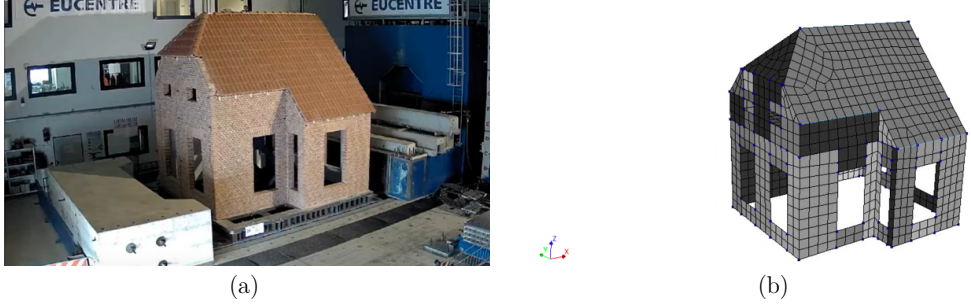
Figure 7.2: Real EUC-BUILD2 prototype (a) and realized numerical model in DIANA FEA (b).
