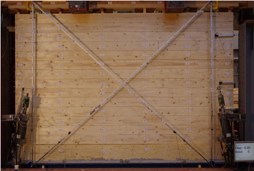
Figure 3.5: Schematic representation of the diaphragms tested perpendicular to the joists (specimens DFper-3 and 3s, DFper-4 and 4s, view from decking side); (b) sample DFper-3 positioned in the test setup.
