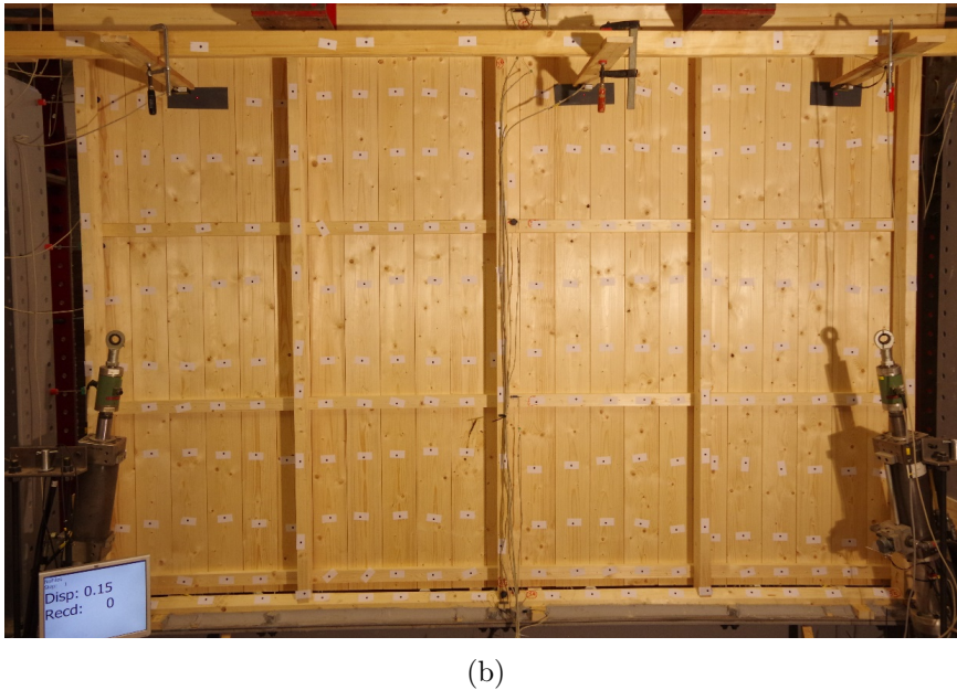
Figure 3.6: Schematic representation of the tested roof pitch (specimens DFpar-5 and 5s, view from the inner side); dimensions in mm; (b) sample DRpar-5 positioned in the test setup.
